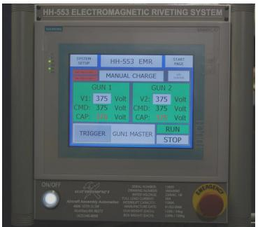
Figure 6 - Siemens Touchscreen PLC
