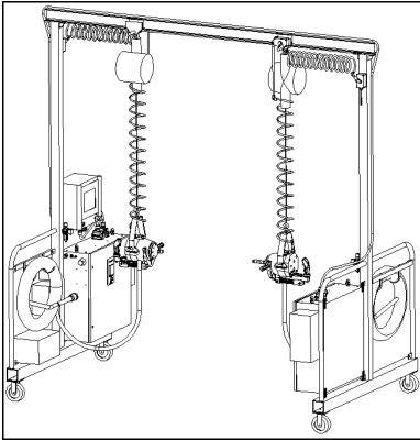
Figure 1 - HH-553 Riveting System
