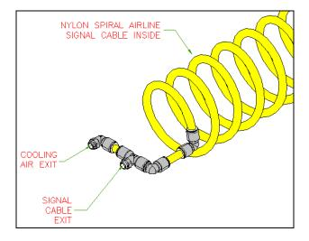
Figure 4 – Air-Signal Segment (Actuator end)
