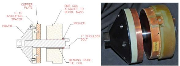
Figure 3 – Center-less Coil Driver Assembly
