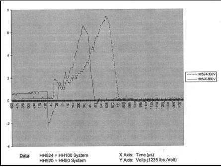
Figure 5 - 500V vs. 1000V EMR Comparison
