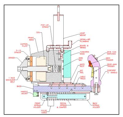
Figure 2 - HH-553 Actuator Cutaway Diagram
