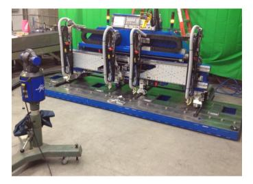
Figure 20: Laser tracking alignment plate bushings with machine mass positioned on plate.
