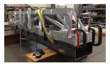
Figure 6: Main machine frame prior to first stress relieve operation.
