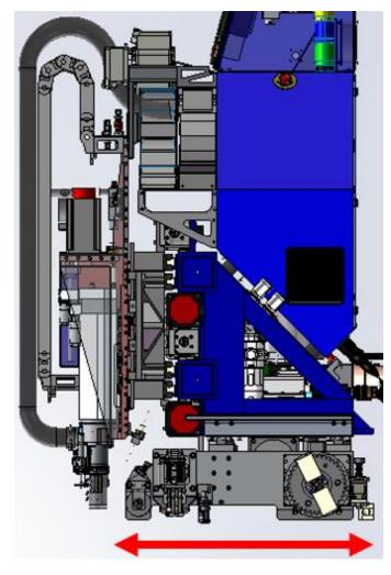
Figure 4: Frame width in X was limited due to proximity of floor grid holes relative to edge of grid.
