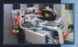
Flextrack CNC ultralight drilling machine adapts to curved surfaces
