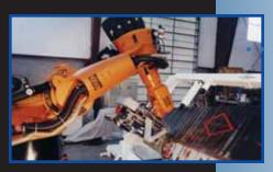
Electroimpact end effector on KUKA robot enables aircraft quality hole drilling
