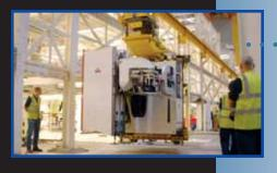
HAWDE CNC drilling machine travels up and down elevators and moves between jigs
