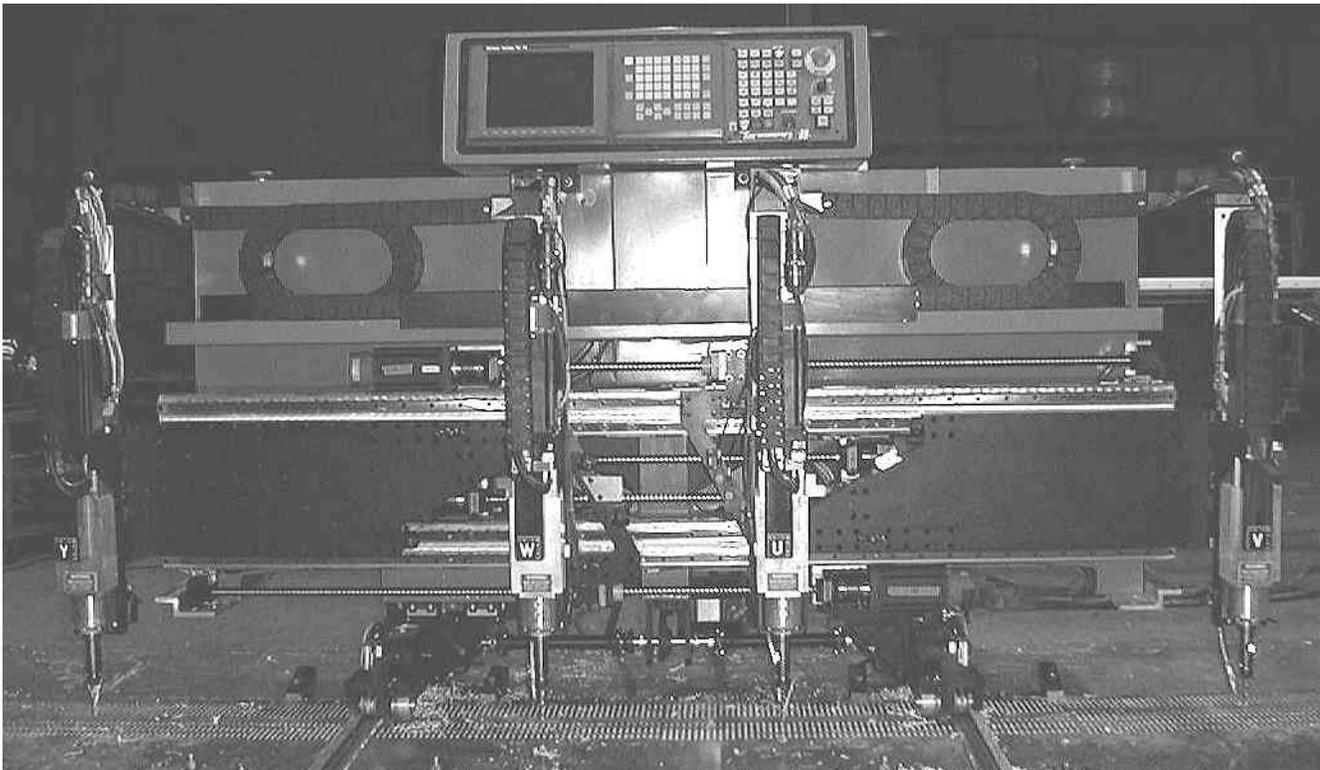
Figure 1: Front photo of AFDE2 showing CNC monitor and drills
