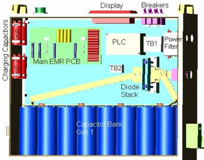
Figure 4. Control/capacitor box
