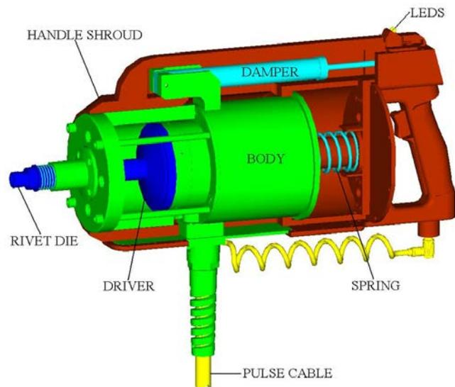
Figure 2. HH503 actuator cutaway
