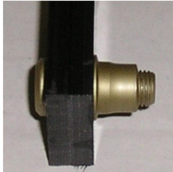
Figure 1 – 3/8 Pin with CT collar in graphite stack.
