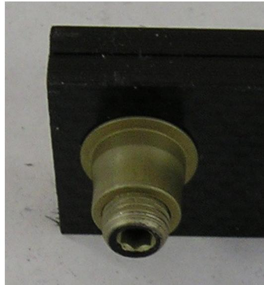
Figure 2. Tail view of 3/8 pin with CT collar
