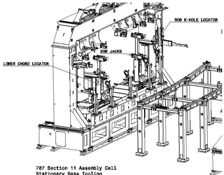
The Lower Chord tooling indexes and clamps the Lower SOB chord in position, while allowing each individual index to be either dropped for access, or indexed at an offset for inspection measurement. The SOB Ribs are indexed using an air powered jacking system and aligned with pins through the coordination holes. The stationary base also provides access at an optimum work height for technicians, as well as easy access to the inside of the Section 11.
