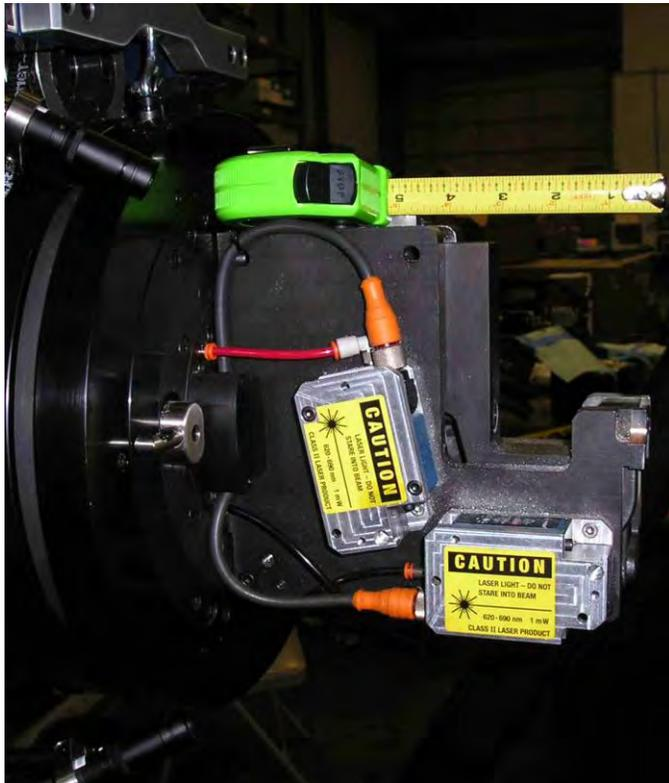
**Figure 9 Stringer side EMR offset anvil with laser**
