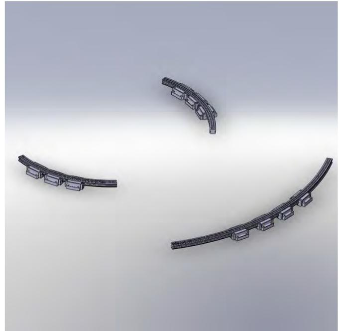
Figure 6 - B axis bearing arrangement
