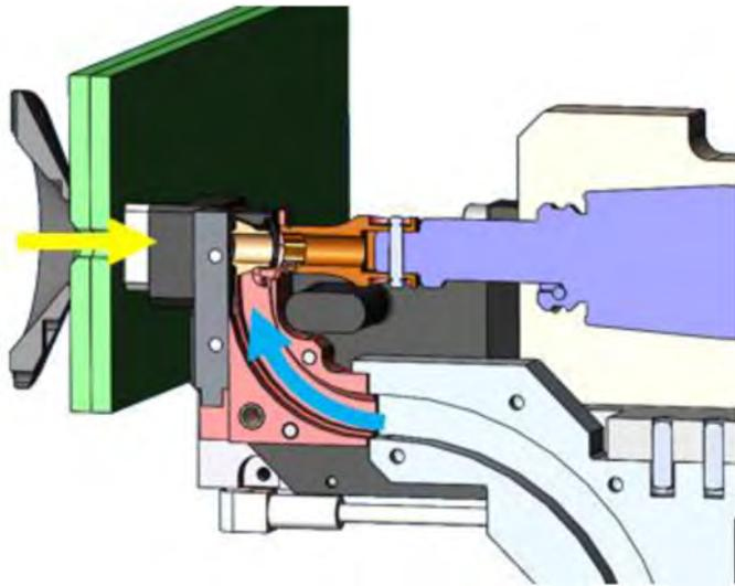
Nut Cycle Step 2. Drill and countersink hole, feed nut.
