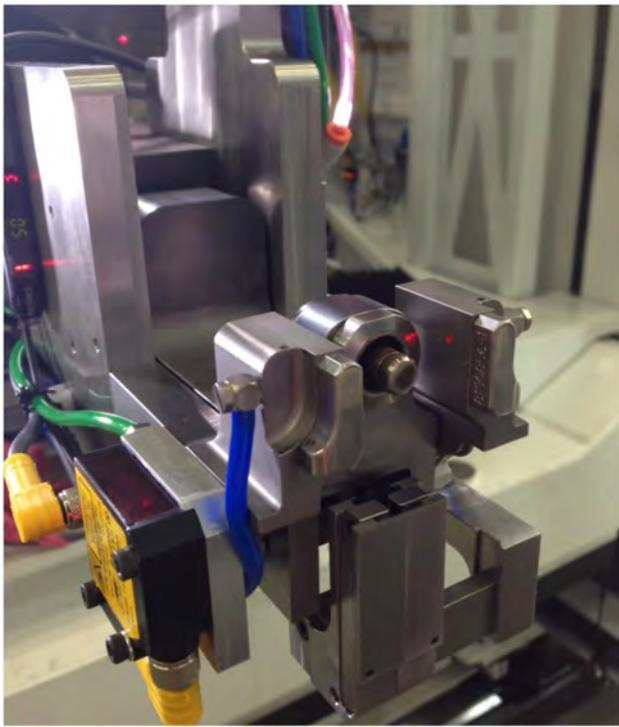
Figure 5. Offset collar anvil with active ram extended and loader visible below
