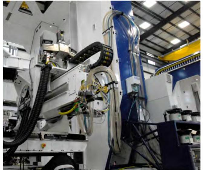
Figure 4. LGP collar and TN nut feed path shown with buffers and vibratory bowls
