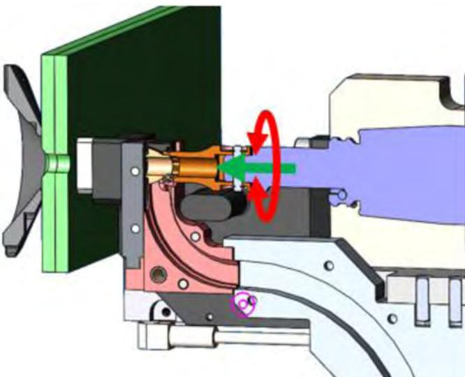
Nut Cycle Step 3. Machine drives forward while spindle performs ample routine, engaging 12-point pattern with socket and retaining spring. Rod lock is actuated while bolt is fed.
