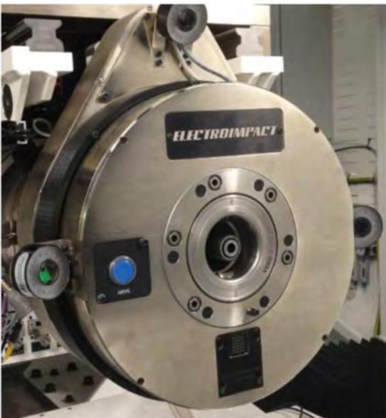
Figure 3. Stringer side process head with clamp cylinder rod visible in center
