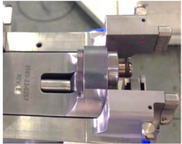
Figure 9. Offset collar tool with active ram retracted
