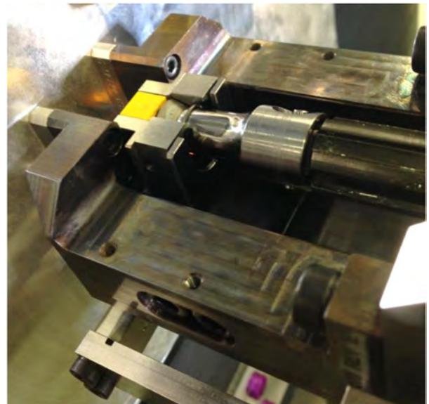
Figure 7. Nut runner socket engaging nut in loader
