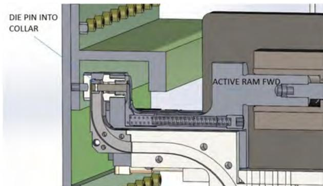
Collar Cycle Step 4. Die pin extended into collar
