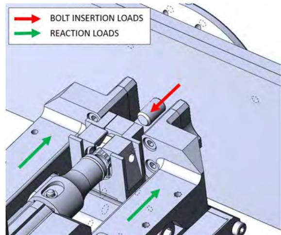
Figure 10. Bolt insertion reaction loads
