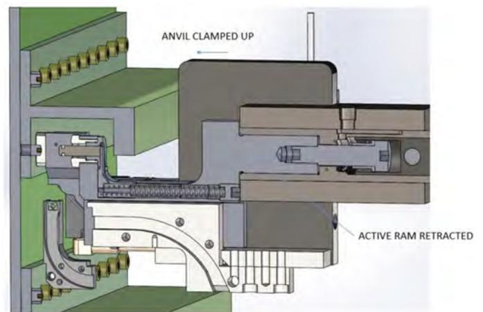
Collar Cycle Step 1. Anvil clamp up, active ram retracted
