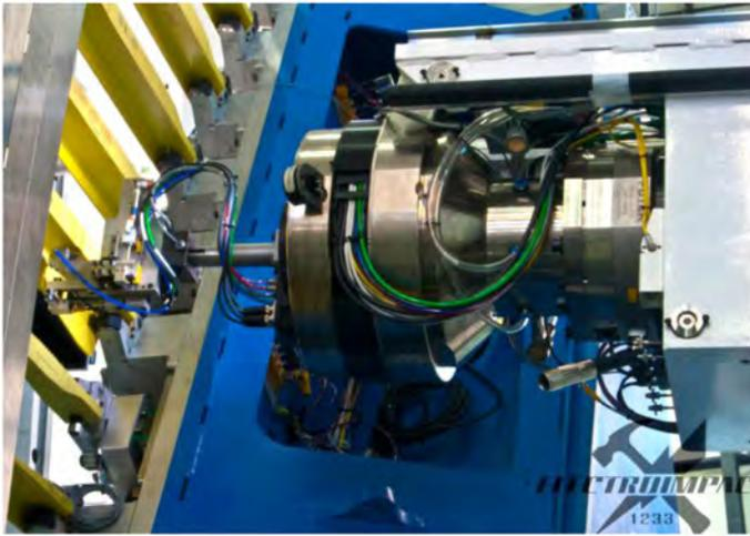
Figure 2. PAL machine navigating 737 stringer with offset tool installed at Electroimpact
