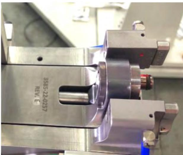
Figure 8. Offset collar tool with active ram extended
