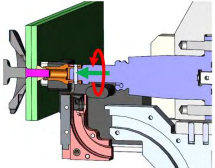
Nut Cycle Step 5. Spindle runs nut down Hi-Lok threads and torques to specification. Machine unclamps.
