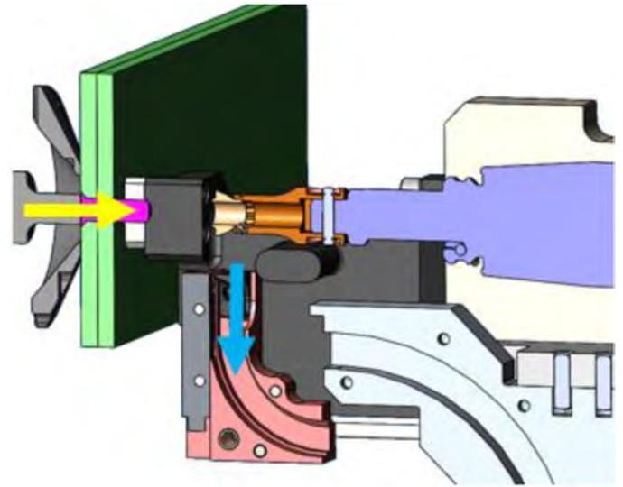
Nut Cycle Step 4. Socket strips fastener from loader fingers as loader retracts. Hi-Lok is inserted and rod lock is released.
