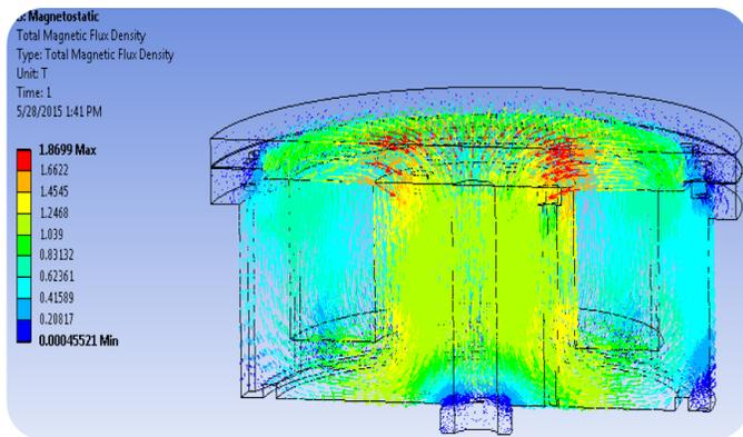
Figure 11. Magnetic flux density analysis
