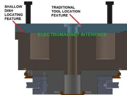
Figure 8. Shallow locating bore detail
