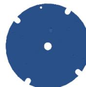
Figure 10. Shoulder screw slots on baseplate
