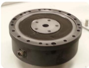
Figure 7. Electromagnet base
