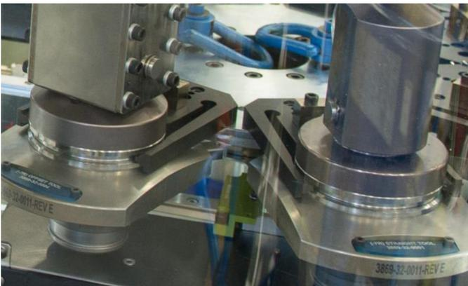
Figure 4. ATC grippers and tool interface
