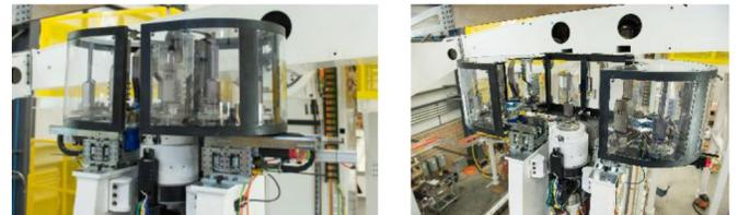
Figure 6. ATC compact vs. expanded orientation.
