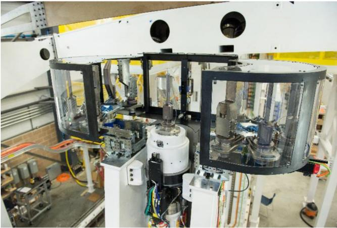
Figure 3. ATC and lower fastening head below test panel
