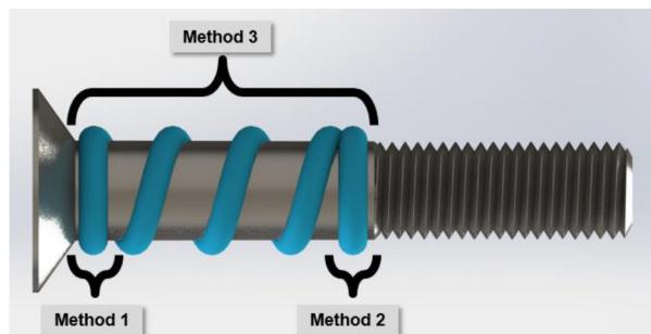
Figure 5. Sealant Methods
