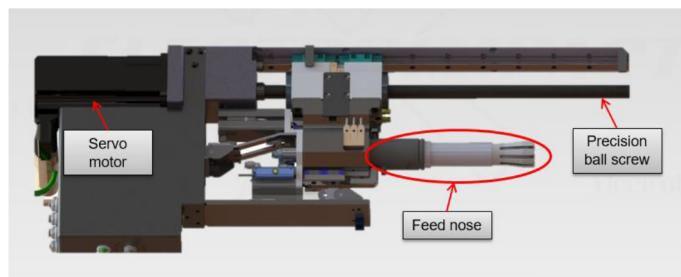
Figure 4. Servo-driven bolt inserter
