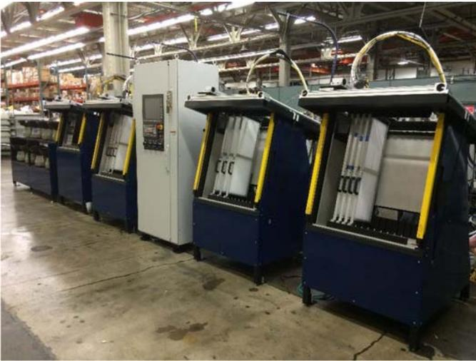
Figure 2. Off-Line Cartridge Filling Station
