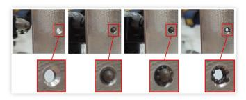
to implement a special 'sealant check' step at this point in the process to confirm full coverage.
