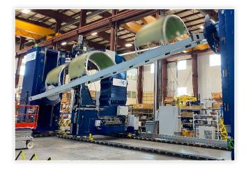
of fastening different types of aircraft parts. Customer requirements also necessitated that the positioning system exhibited the capability of holding an entire shipset (4x fan cowl doors) at once.
