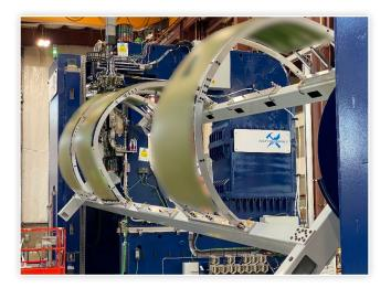
**FIGURE 3** Machine Design Phase Access Study - Panel positioner was overlayed in CAD in many different positions to form a "design constraint cloud" which informed the shape of the lower portion of the fastening machine.
