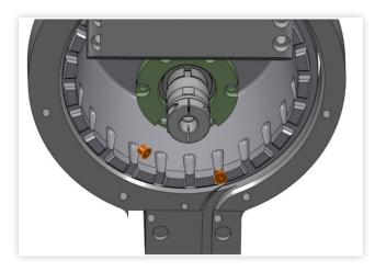
reliably without jamming by using a mechanical poka-yoke gate (Figure 13) that does not allow the fasteners to escape the drum unless they are in the correct orientation. Once the fasteners leave the drum, they are fed into a small buffer rack. A sensor on the buffer rack triggers the control system to rotate the drum to refill it when necessary. The entire assembly is mounted directly on the OML process head of the machine, so the fasteners do not need to be fed in tubes.
