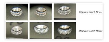
and that process parameters that resulted in heavier chip loads were likely the reason(s) for these results.
