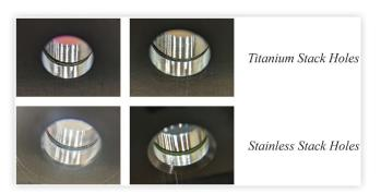
**FIGURE 7** Exit burrs are automatically removed by the fastening machine using an IML-side cutter. The machine is programmed such that the cutter barely makes contact with the material in this process.
