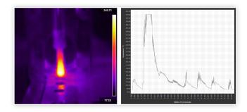
frequent pecking and re-lubrication, but this also slowed the process down considerably. To overcome this, a thermal imaging camera was utilized to collect data, which informed where and how pecking could be reduced while keeping cutter temperature(s) as low as possible.
