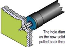
The hole diameter is expanded as the now solidified mandrel is pulled back through the material.
