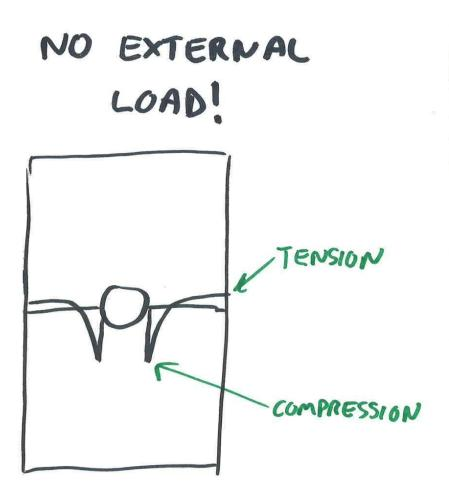
It has a locked in compressive stress at the edge of the hole, perfect for counteracting the higher stress at the edge of the hole from external loading. Combining the 2 states of stress, we get a more even
