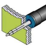
Pass-thru is complete. Nosecap is placed flush to material. After depressing trigger, the pilot extends through center of hollow mandrel, which solidifies.
