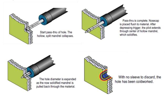
Boeing became the largest user of split mandrel coldworking, processing millions of holes starting in the 1980's – generally in lower panel wing skin to spar joints or lower wing skin splices.
