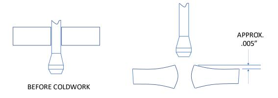
On the one hand, the volcano regains a little bit of cross section of material so there is a slight reduction of stress near the hole. On the other hand, the part is now around .010" thicker than it was near the hole – so for a multi-part stackup, you can gain a fair amount of thickness in the vicinity of a coldworked hole. The volcano can be machined or sanded off with little effect on fatigue life, but then maybe you
