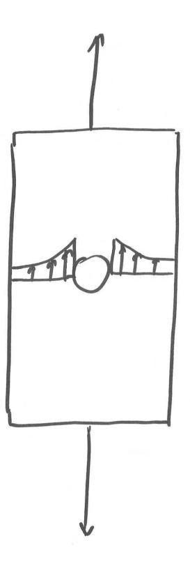
This is bad – a 20% increase in load will cut fatigue life in half. Enter the coldworked hole with this stress distribution -
