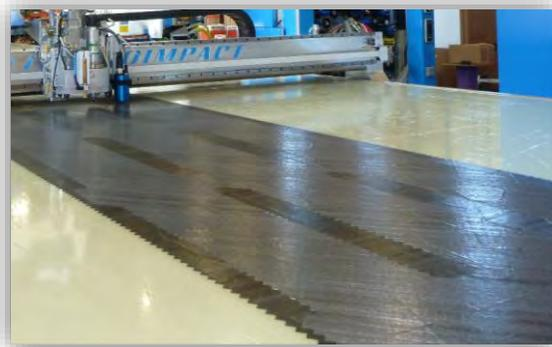
Figure 3: Steered Fiber and Neat Net Shape Layups.
